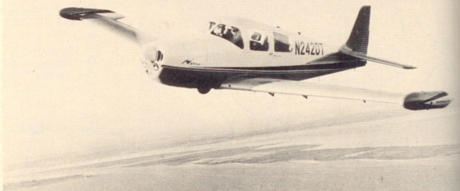
Navion Rangemaster in flight. The Texas-built version of the famed plane, carrying 107.5 gallons of fuel, has a nonstop capability of more than eight hours
